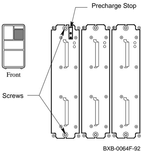
4. When removing a regulator, do not touch the 33-pin DC connector on the rear of the regulator. Cover the charged connector with the conductive foam provided with the replacement regulator to prevent rapid discharge of the stored energy.
