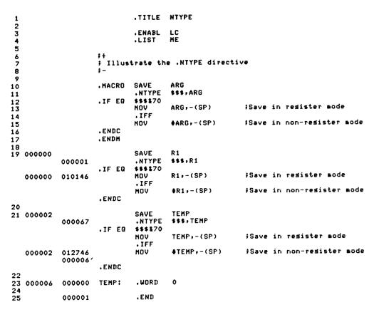
Figure 7-3 Example of .NTYPE Directive in Macro Definition
