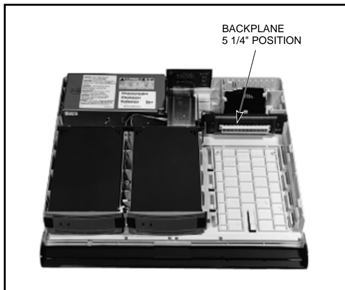
Figure 4-4 Backplane In 5¼-Inch Position
